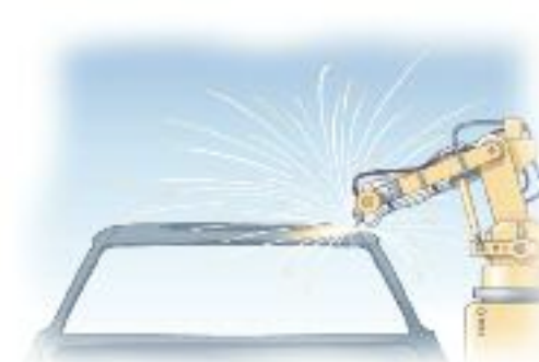
Robot welders, used in car manufacturing, are controlled by computers.
