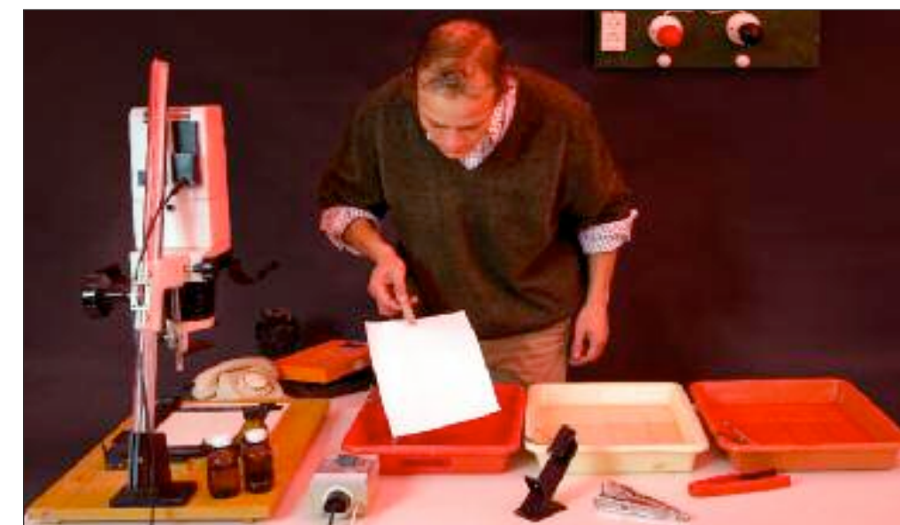
A darkroom showing (from left) an enlarger and trays of developer, stop bath and water.
